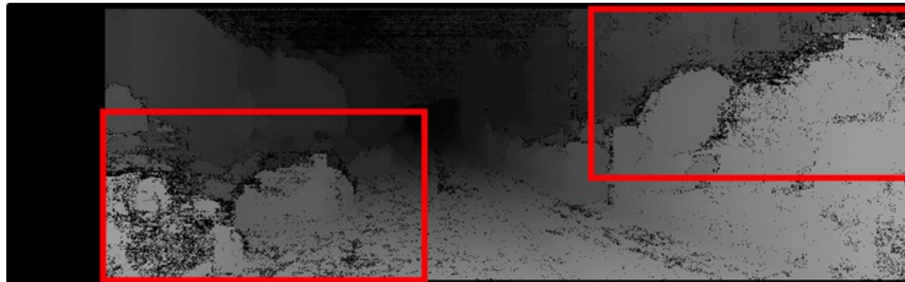
Fig. 1. Initial disparity map using semi-global matching (SGM)
